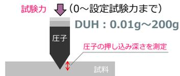
ISO 14577 :2002 Metallic materials - Instrumented indentation test for hardness and materials parameters
